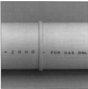
Figure G Correctly Made Butt Fusion Joint
