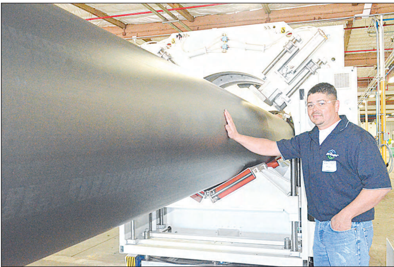
JM Eagle's Michael LaFollette shows those invited to yesterday's open house the pipe cutter used to cut 36-inch pipes to length.
