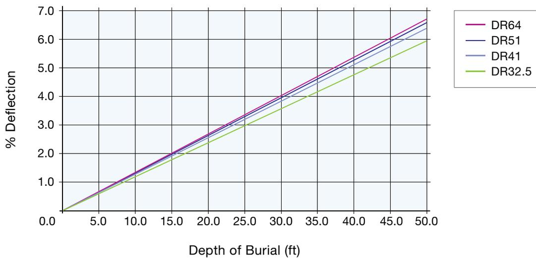
:: Deflections computed using a unit weight of backfill at 120 lbs/cft and assume no internal pressure or live load.
