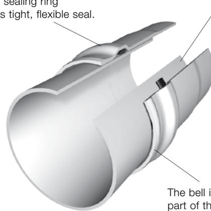
The bell is an integral part of the pipe length with the same strength.
